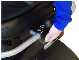
Lift black lever on left side.
